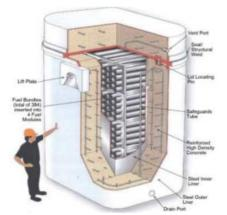
Figure 55: Cutaway view of the concrete cask developed by OPG
