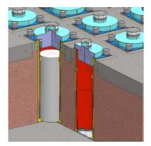
Figure 27: Cutaway view of the HI-STORM UMAX concept
