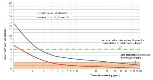
Figure 4: Cooling period necessary before dry storage, for fuels irradiated in a PWR in France
