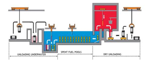
Figure 5: Principle of unloading the fuel underwater or in dry conditions
