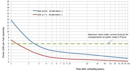
Figure 1: Curves for decay of the residual heat of a UOX fuel assembly and a MOX fuel assembly irradiated in a PWR in France
