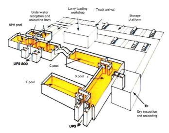
Figure 14: Schematic diagram of the layout of the spent fuel pools on the Orano Cycle site at La Hague
