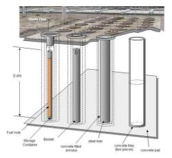
Figure 30: Cutaway view of the WMA 'B' facility at Chalk River (Canada)
