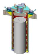
Figure 28: Cutaway view of a cavity of the HI-STORM UMAX concept
