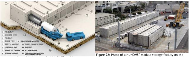
Figure 21: Diagram of a NUHOMS® module
