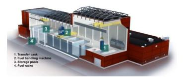
Figure 8: Cutaway view of the spent fuel pool known as TVO-KPA-STORE (Olkiluoto site, Finland)
