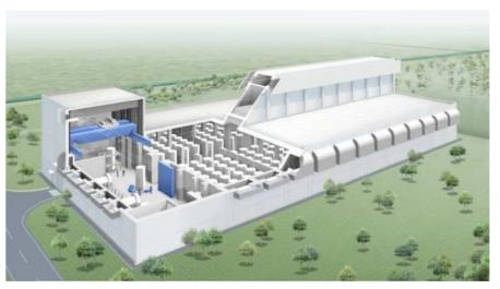
Figure 71: Cutaway view of the future centralised storage facility at Mutsu (Japan)
