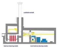
Figure 62: Cross-sectional view of the HABOG facility (Borsele - Netherlands)
