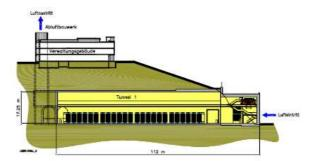
Figure 51: Cutaway view of the tunnel storage facility at Neckarwestheim (Germany)
