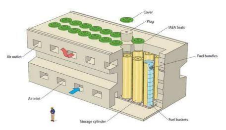
Figure 23: Cutaway view of the MACSTOR® storage facility concept
