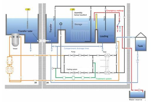
Figure 7: Cutaway view of the reactor cavity in the reactor building (BR) and the spent fuel pool in the fuel building (BK)
