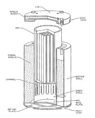
Figure 31: Cutaway view of the HI-STORM 100 concept
