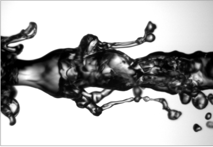
Figure 5.30. Illustration of fragmentation process complexity in the case of a liquid jet in a coaxial air flux [63].
