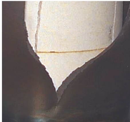
Figure 5.9. Overview of the burst in tube no. 2 in 316L steel with a temperature ramp of 0.05\text{ }^{\circ}\text{C/s} and a membrane stress of 107 MPa.
