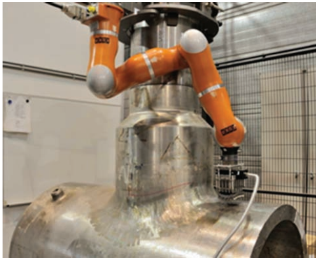
Figure 10.8 Examination of a nozzle with a conformable transducer (2014 Cofrend Conference – Strategy for robotized examination of nuclear components: from examination design to experimental results). © CEA.
