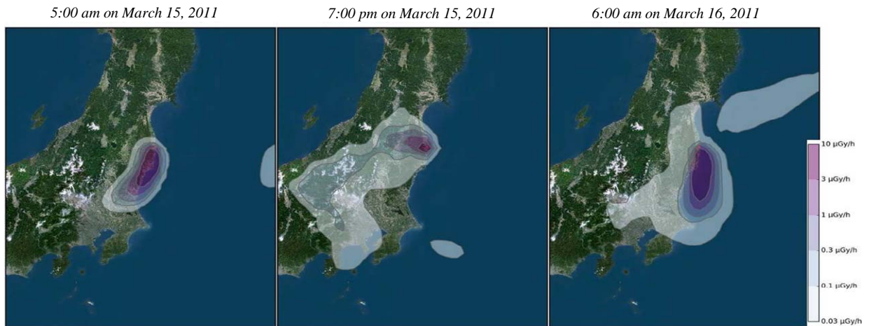
Figure 6-6 - Model of the ambient dose rate due to atmospheric dispersion of releases from the Fukushima accident on March 15 and the morning of March 16 (excluding the contribution of radioactive fallout - IRSN's IdX model), illustrating the first air contamination event on Honshu island.
