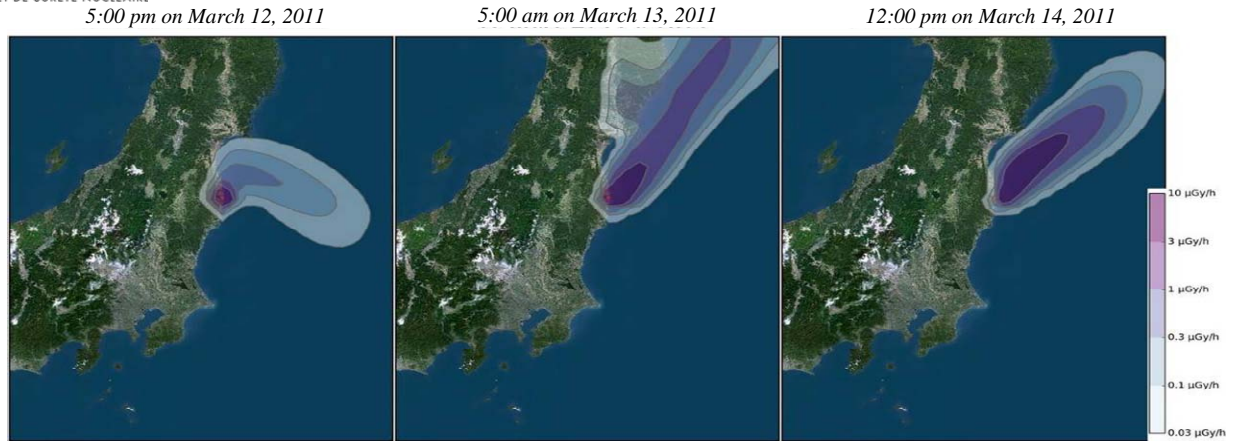
Figure 6-5 - Model of the ambient dose rate due to atmospheric dispersion of releases from the Fukushima accident between March 12-14 (excluding the contribution of radioactive fallout - IRSN's IdX model).
