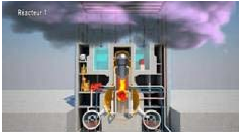
Figure 5-6 - Schematic diagram of the explosion in reactor building 1
