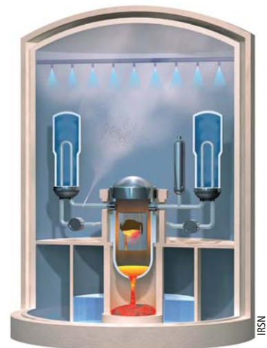
Astec software simulation of a core meltdown accident in a pressurized water reactor.
